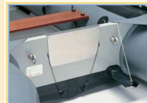
HEAVY-DUTY SELF-BAILER AND ALUMINUM-PLATED TRANSOM.
