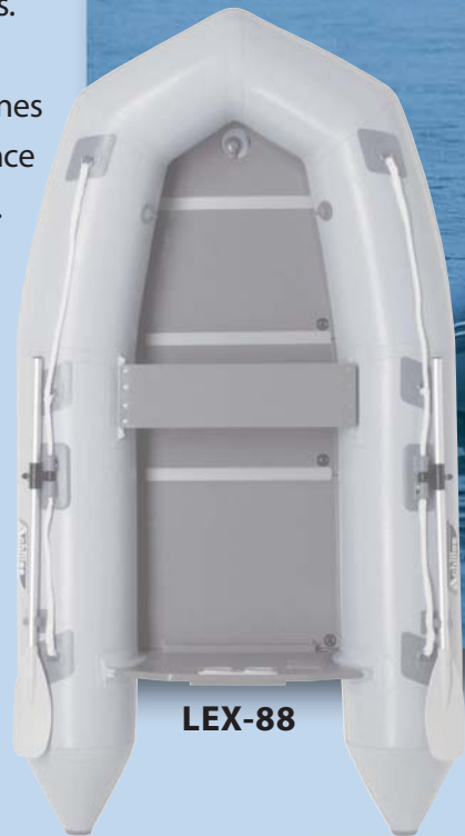
Painted marine grade floorboards, seat and transom
